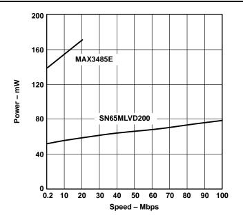
Figure 2. Power Versus Speed for SN65MLVD200 and MAX3485E
