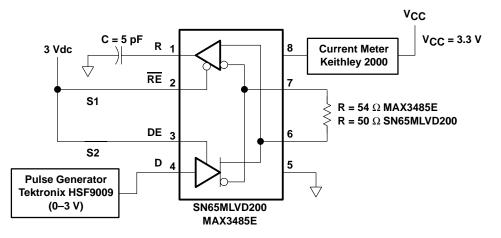
Figure 3. Test Setup
