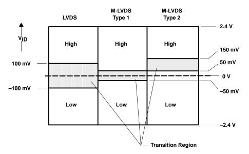
Figure 3. Differential Input Voltage Threshold Comparison
