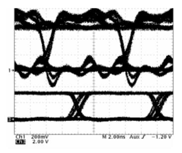
Figure 6. Eye Patterns at Node 2 With 100-Mbps PRBS Into Node 1
