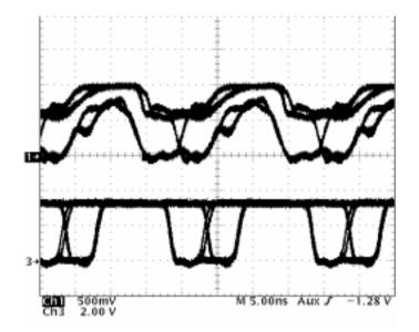
Figure 13. Eye Patterns at Node 4 With PRBS Into Node 3 and Pulse Into Node 1
