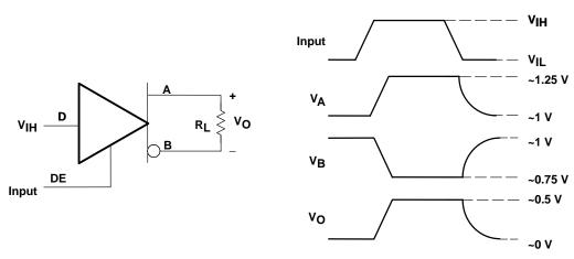
Figure 2. Wired-OR Operation of M-LVDS Driver
