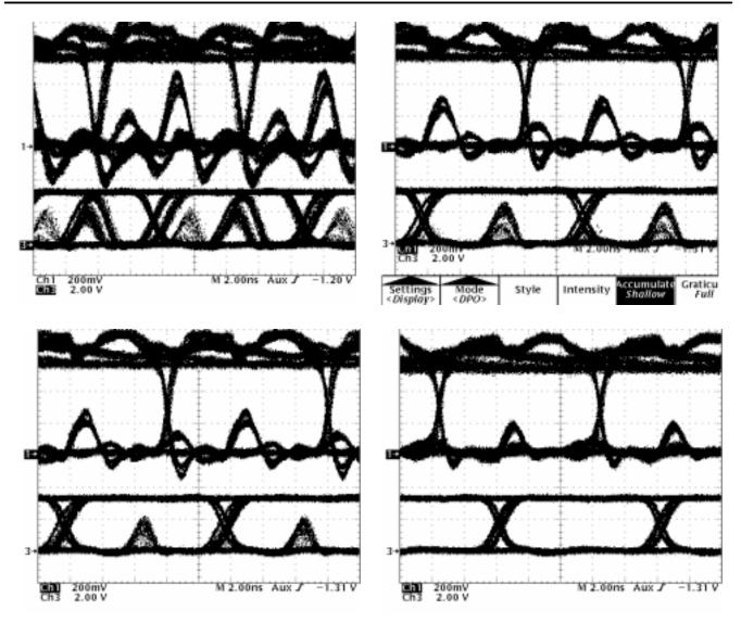
Figure 14. Eye Patterns Into and Measured at Node 3 as Capacitance Decreased
