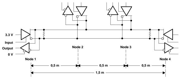
Figure 4. Test Bus Schematic Diagram
