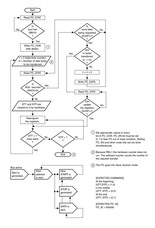
Figure 11. Master Transmitter Mode, RM = 1
