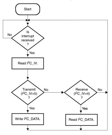
Figure 21. Slave Transmitter/Receiver Mode-Interrupt
