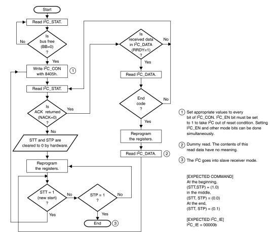
Figure 13. Master Receiver Mode, RM =1, Polling 2 (Number of the Receive Data is Variable, Data Contents Dependent)
