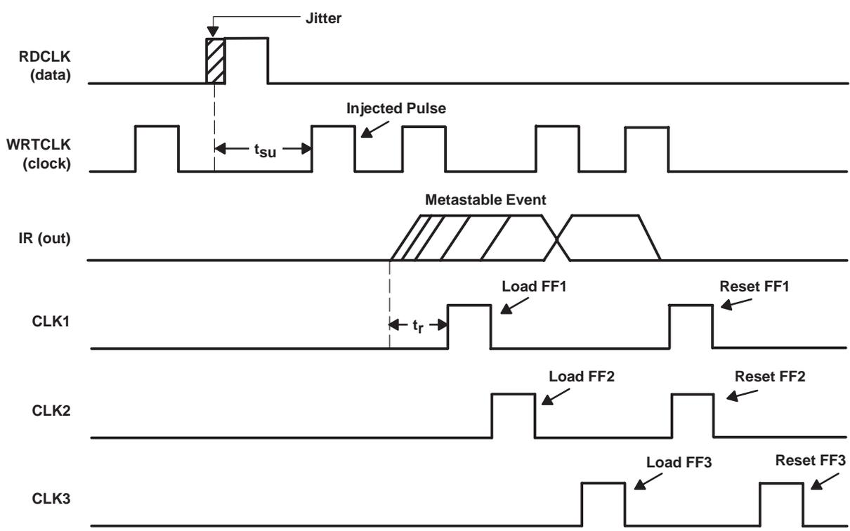
Figure 4. Metastable Event Counter and Input Waveforms
