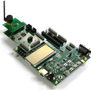
Insert a CC2520EM into both the SmartRF05EB's. The connectors will only fit in one position. Connect antennas to both of the CC2520EM. Insert this board into the CC2520EM. These connectors will also fit in only one position. Do not force the boards.
