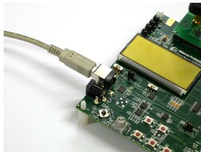
The SmartRF05EB can also be powered from the USB cable.
