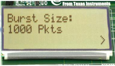
Select burst size by navigating the joystick, either 1000, 10K, 100K or 1M packets. Confirm the selection with Button 1.
