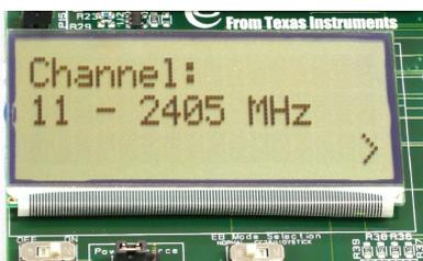
Select a channel between 11 and 26 (2405-2480 MHz). The channel is selected by navigating the joystick to the right or left. Confirm the selection by pressing Button 1.
