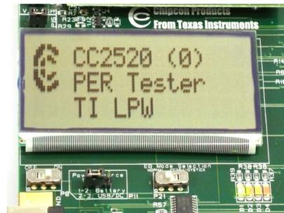
When power is applied to the board set the power switch in the ON position and the PER test program will start. The LCD will display the screen as shown in the picture above. Press Button 1 to enter the menu.
