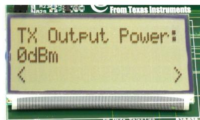
On the transmitter node, selection of TX output power and burst size (number of packets to send) is also needed. Select TX output power by navigating the joystick, either -4 dBm, 0 dBm or 4 dBm, and confirm with Button 1.
