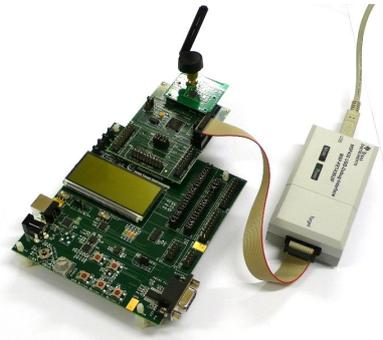
In order to program the MSP430 MCU on the CCMSP-EM430F2618 board the MSP430 Debug Interface is needed. Connect the MSP430 debug interface to JTAG connector P12 on the CCMSP-EM430F2618. Connect the debug interface to the PC with a USB cable.
