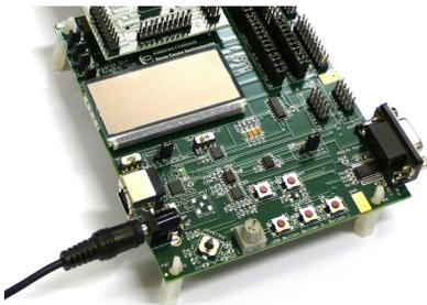
Alternatively a 4-10V DC power source using the jack connector can be applied. The centre pin is + and the sleeve is connected to ground. Set the power source jumper on the EB in position USB/DC.
