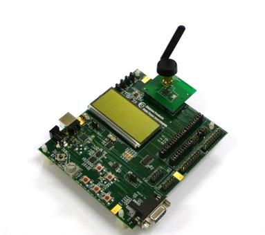
In order to use the SmartRF Studio the CC2520EM is connected directly to the SmartRF05EB.
