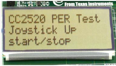
The transmitter is now configured for the PER test. The PER test is started by moving the joystick UP. The transmitter will display the number of packets sent during the PER test. The PER test is stopped by moving the joystick UP again.
