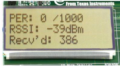
The PER test receiver will display the total PER (calculated based on the received sequence numbers), and moving average RSSI value on the display. It will also display the number of packets received during the PER test.
