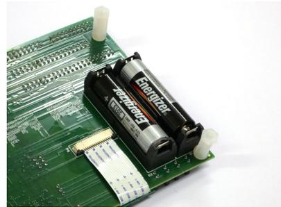
There are three different ways of applying power to the SmartRF05EB. The first method is to insert 2 AA batteries to the battery connectors underneath the board.
