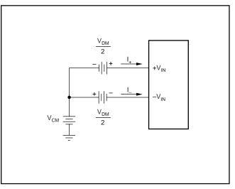
FIGURE 5. Differential and Common-Mode Signal Definitions.
