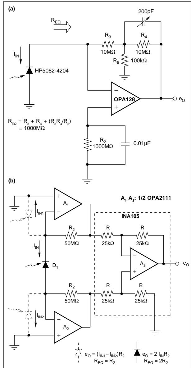
FIGURE 2 (a) Using a T-Network to Design the Feedback Resistor for a Transimpedance Circuit.
