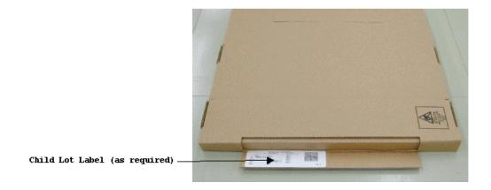
Figure 40. Child-Lot Label Placement on Shipping-Box Label Flap
