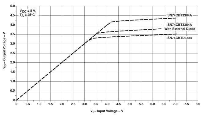
Figure 4.  $V_O$  Versus  $V_I$  of SN74CBT3384A, SN74CBT3384A With 1N916 External Diode, and SN74CBTD3384
