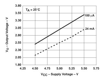
Figure 5.  $V_O$  Versus  $V_{CC}$  of the SN74CBTD3384
