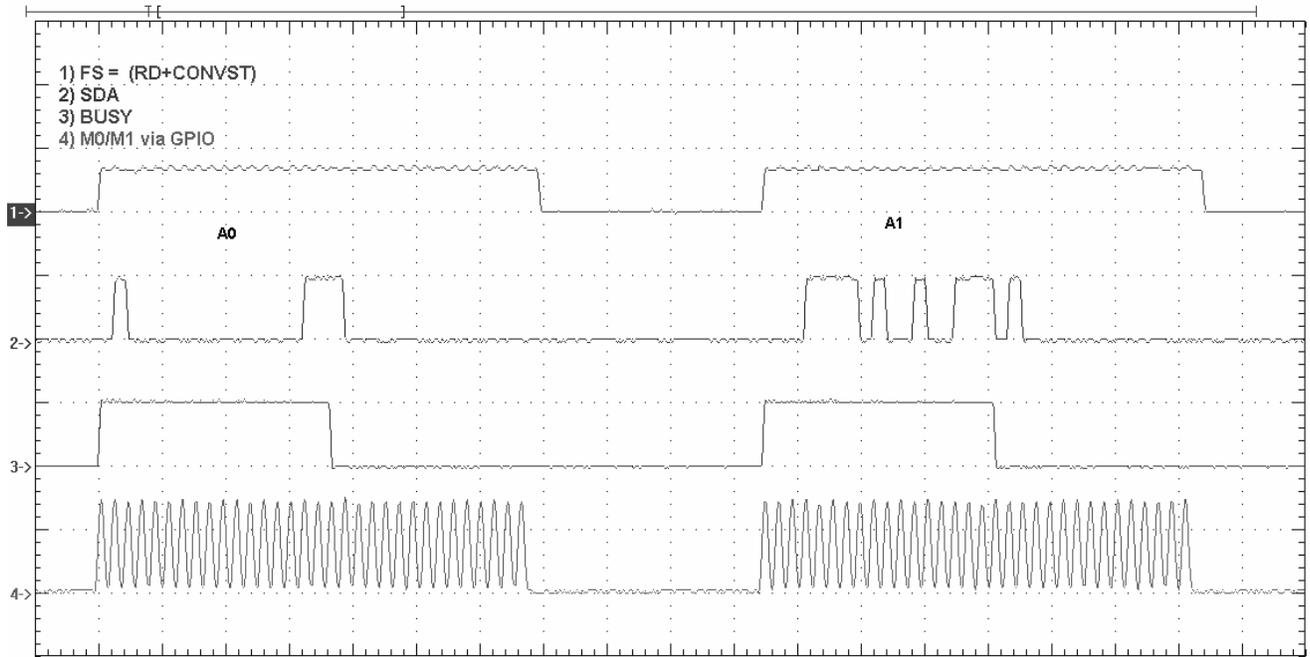
Figure 6. Mode I Waveforms Using McBSP and SPI
