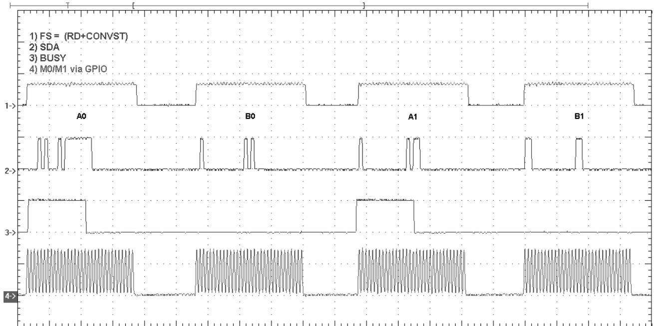
Figure 7. Mode III Waveforms Using McBSP and SPI
