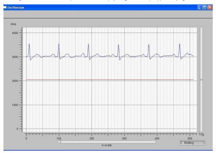
Figure 9. PC Scope Program EKG Display
