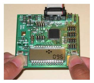
Figure 8. Picture of EKG Board in Action
