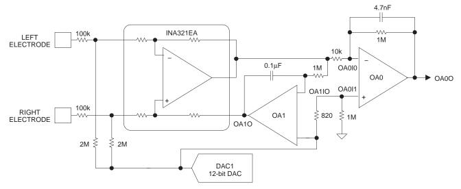
Figure 2. EKG Amplifier Circuit Diagram
