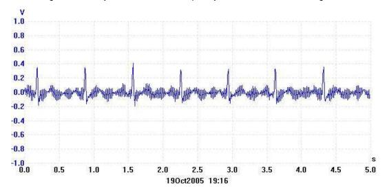
Figure 3. 500× Amplified EKG Signal With 60-Hz Noise Content
