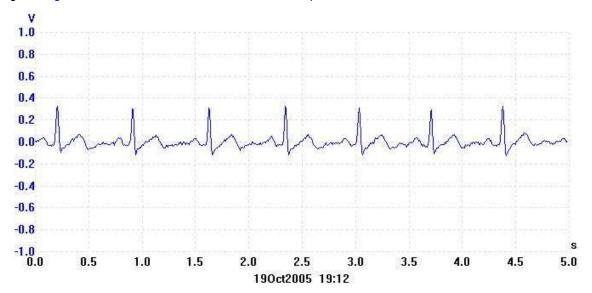
Figure 4. Low-Pass Filtered Waveform at DAC0 Output
