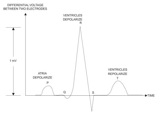
Figure 1. A Typical EKG Waveform
