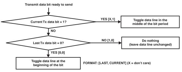
Figure 6. Miller Encoding Scheme Flow Chart
