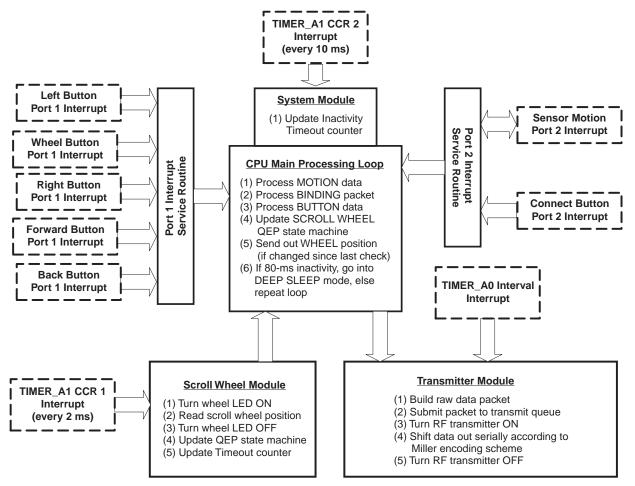
Figure 4. Mouse Transmitter Software Flow Diagram
