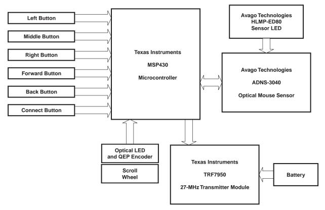
Figure 1. Mouse Transmitter System Block Diagram
