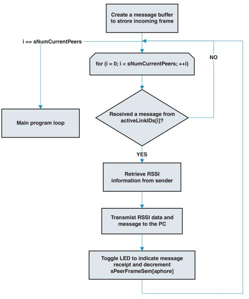
Figure 4. Flowchart for Peer Frame Handling
