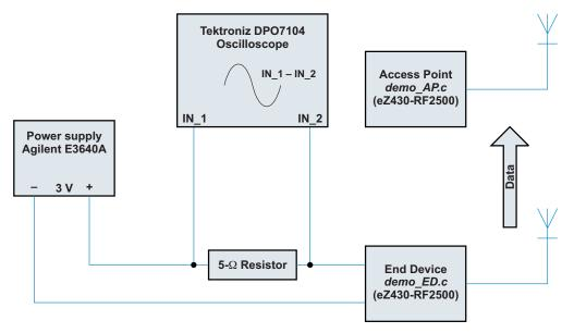
Figure 6. End Device Test Platform
