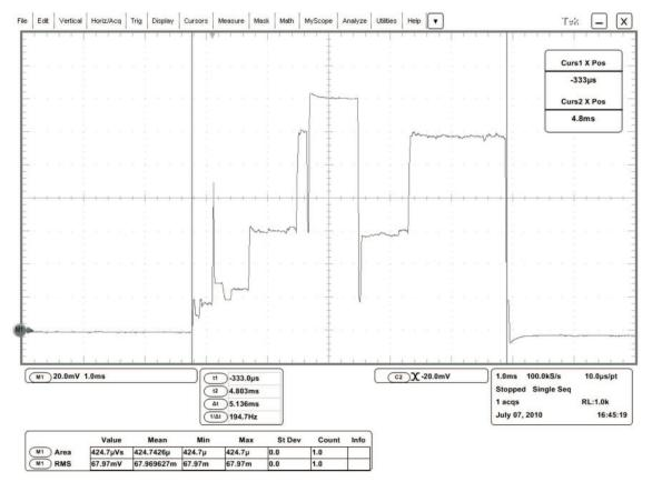
Figure 9. End Device Transmission Current Profile (AP ACK Enabled)
