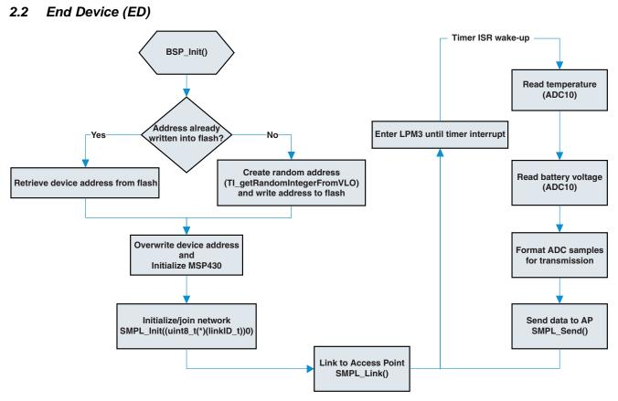
Figure 5. Flowchart for demo\_ED.c
