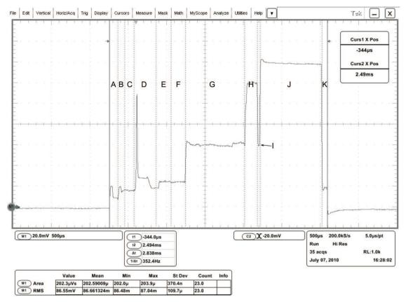
Figure 8. End Device Transmission Current Profile (AP ACK Disabled)
