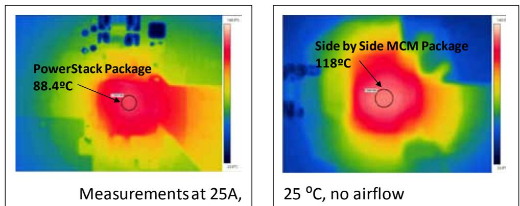
Figure 8: Thermal measurements comparing PowerStack and side by side MCM.
