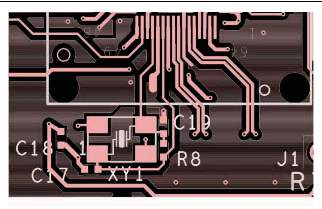
Figure 3. Example Reference Clock Layout
