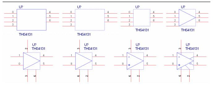
Figure 14. Progressive Steps in Making Part Symbol
