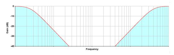
Figure 6. Band Reject Filter
