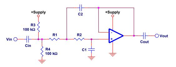
Figure 8. Low Pass Filter for a Single Supply
