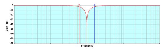
Figure 5. Notch Filter—Single Frequency Rejection
