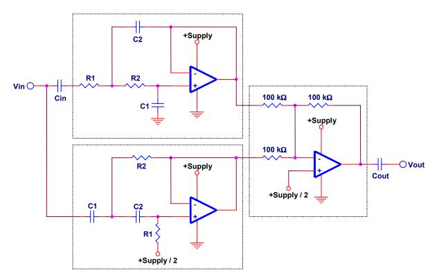
Figure 18. Band Reject Filter for a Single Supply
