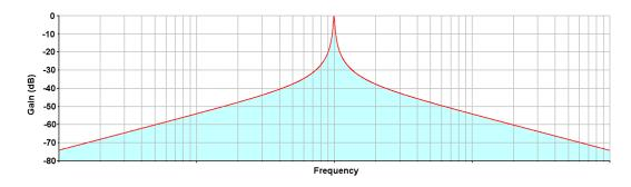
Figure 3. Narrow (Single Frequency) Band Pass—Go to Section 4
