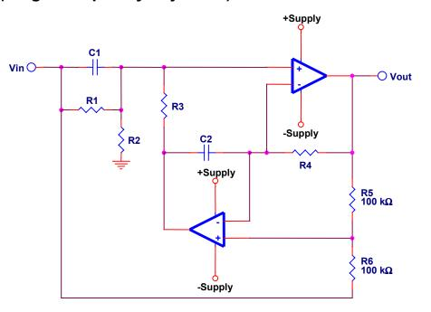
Figure 15. Narrow Band Pass Filter for ± Supplies
