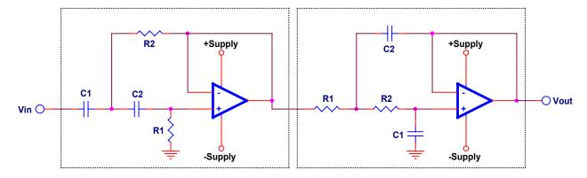
Figure 13. Wide Band Pass Filter for ± Supplies
