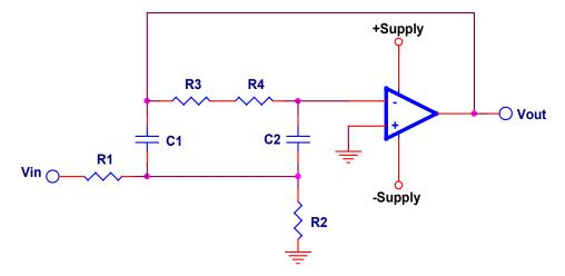
Figure 11. Narrow Band Pass Filter for ± Supplies
