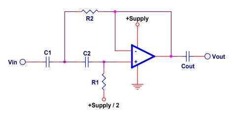
Figure 10. High Pass Filter for a Single Supply
