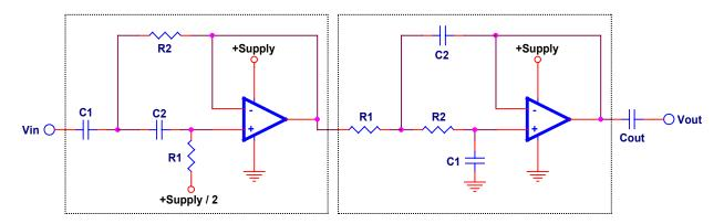
Figure 14. Wide Band Pass Filter for a Single Supply
