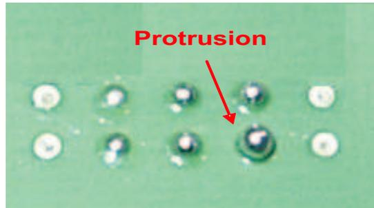
**Figure 7. Protrusion at the Other Side of Board**
