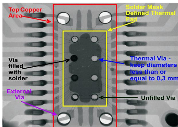
**Figure 5. X-Ray – PCB Device With Internal and External Vias**
