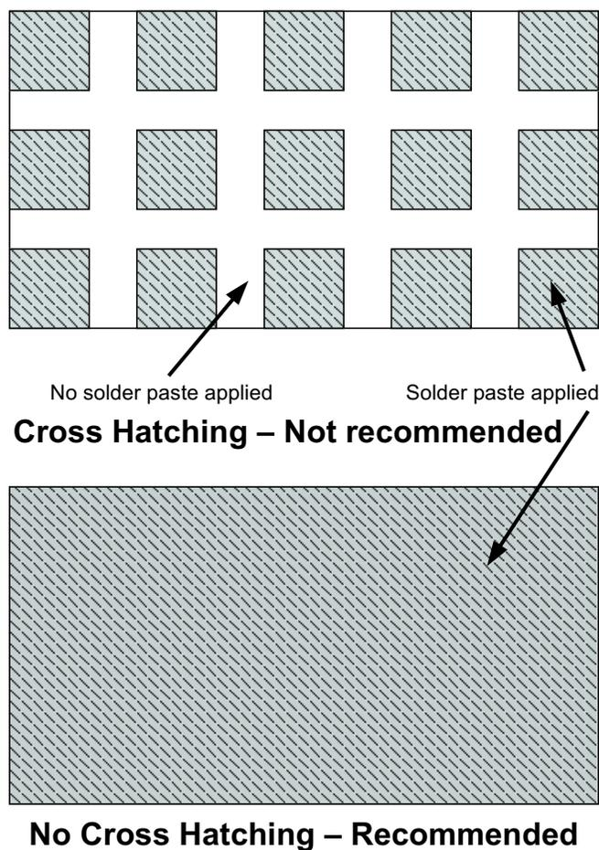
Figure 9. Stencil Thermal Pad Opening
