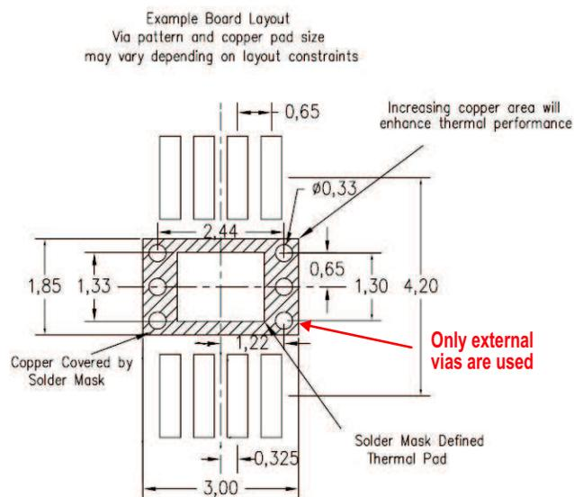
**Figure 6. Example of Using Only External Vias**
