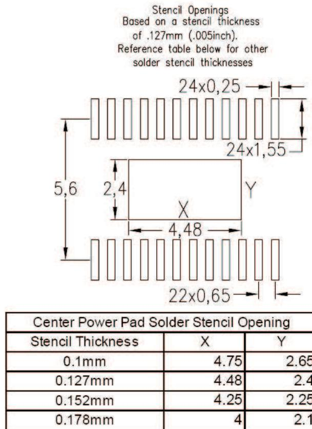
**Figure 8. Recommended Stencil Openings for PCB Package**
