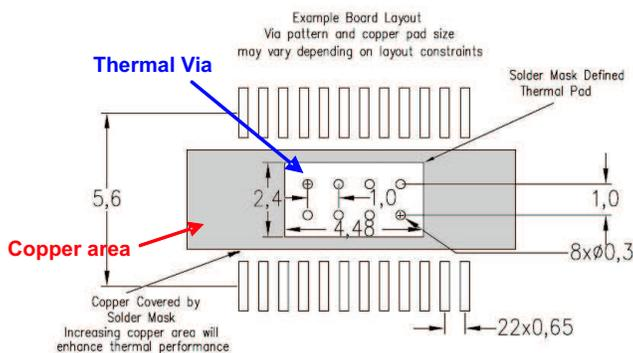
Figure 2. Board Layout for a PCB Package
