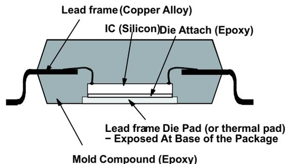
Figure 1. Section View of a PowerPAD Package
