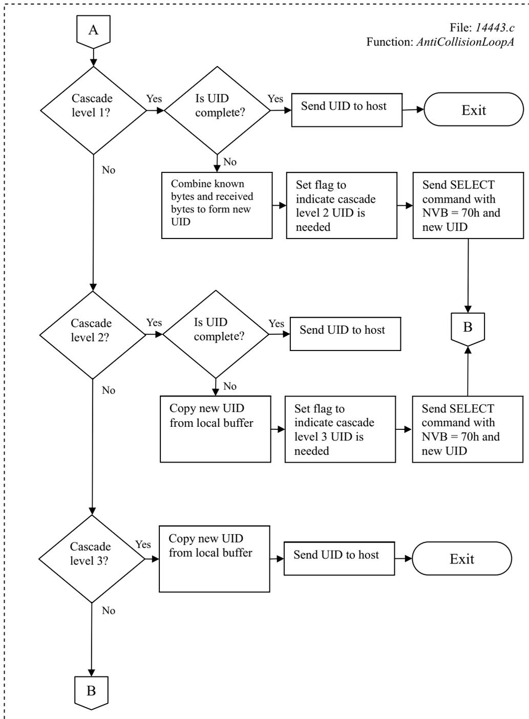
Figure 10. Anti-Collision Loop A (2)
