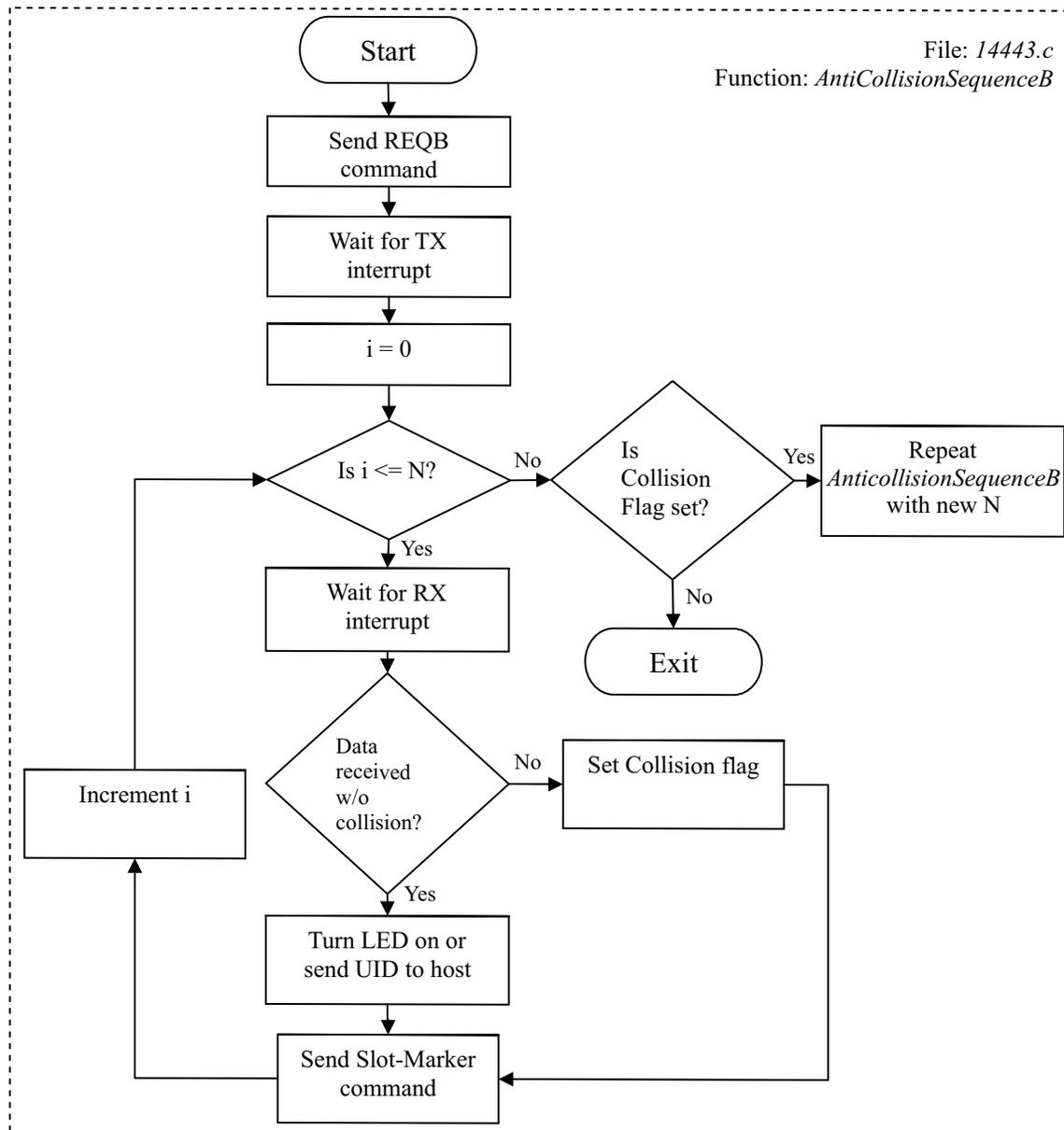
Figure 11. Anti-Collision Loop B
