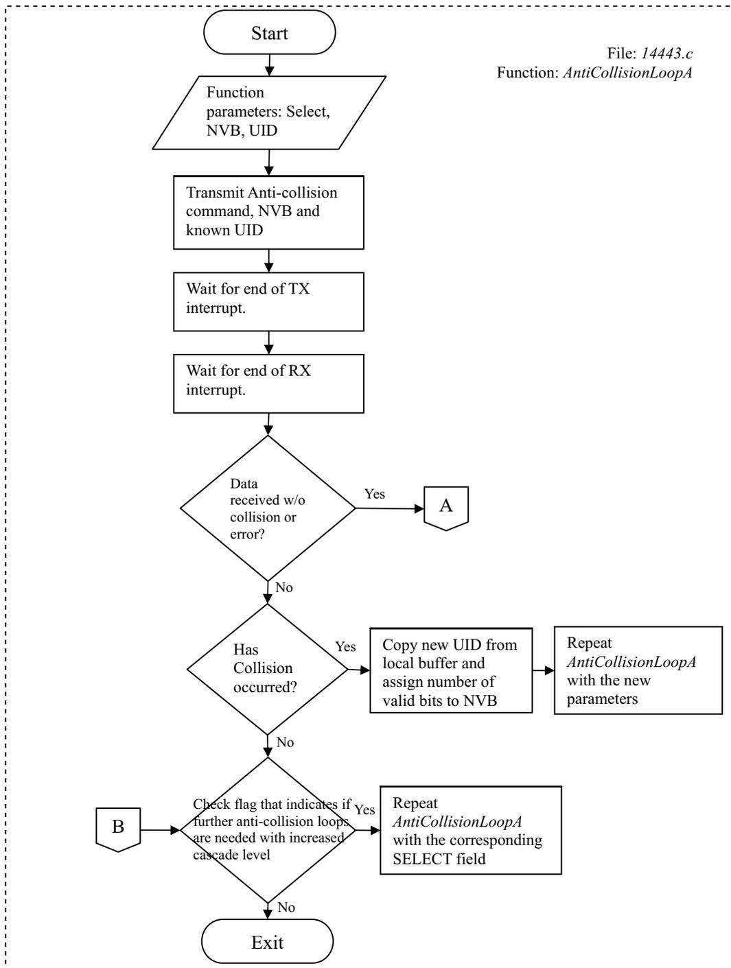
Figure 9. Anti-Collision Loop A (1)
