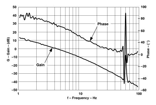
Figure 6. Voltage Loop High-Line Frequency Response at Maximum Load
