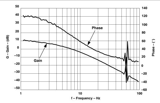
Figure 5. Voltage Loop Low-Line Frequency Response at Maximum Load
