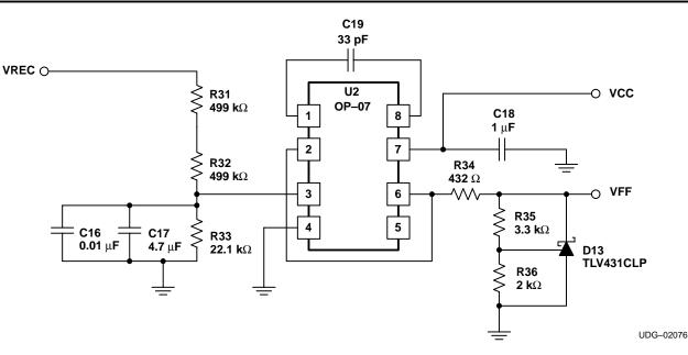
Figure 4. VAI Output Sensing Schematic
