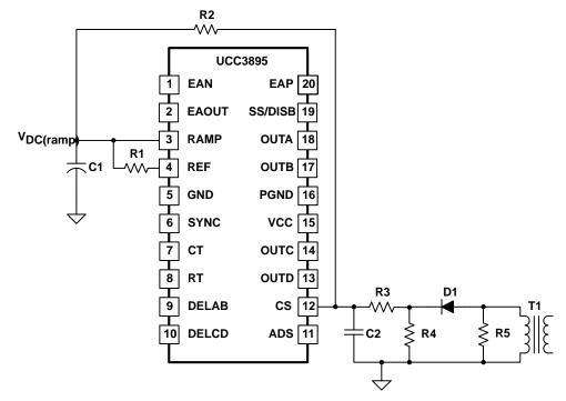
Figure 2. Peak Current Mode Control (slope compensation not shown)
