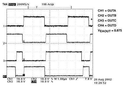
Figure 1. UCC3895 Output Waveforms
