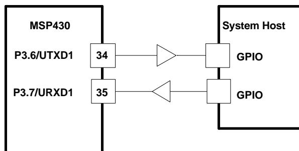
Figure 2. Host Communications Interface (RS-232) Schematic
