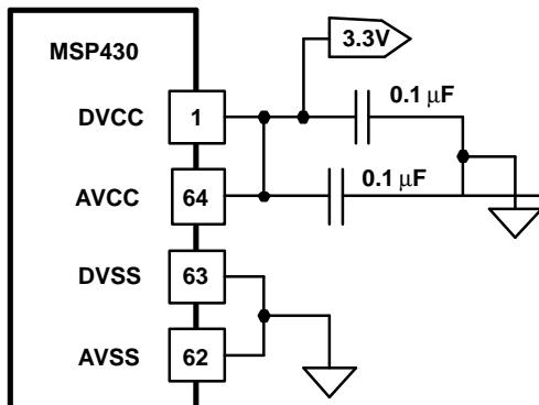
**Figure 9. Power and Ground Schematic**
