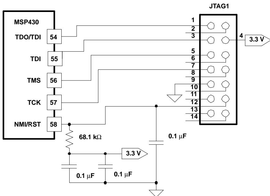
Figure 4. JTAG Interface Schematic
