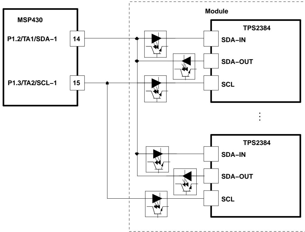
**Figure 3. PSE Communications Interface ( $I^2C$ ) Schematic**
