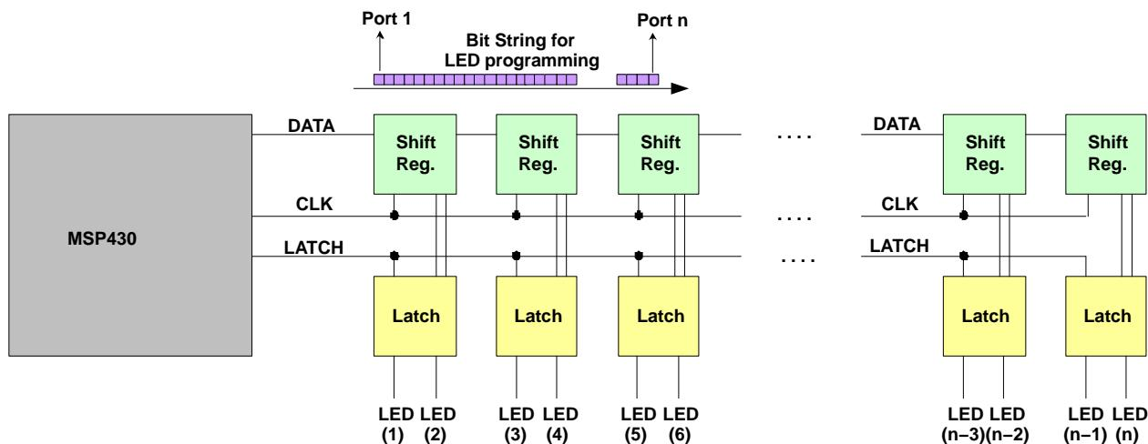
Figure 5. LED Shift Register and Latch Ordering
