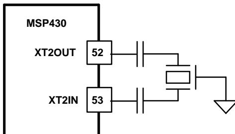
**Figure 8. Clock Circuit Interface**
