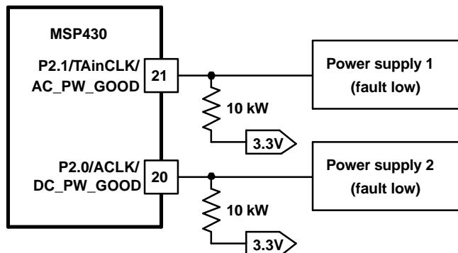
**Figure 7. Power Supply Monitoring Schematic**
