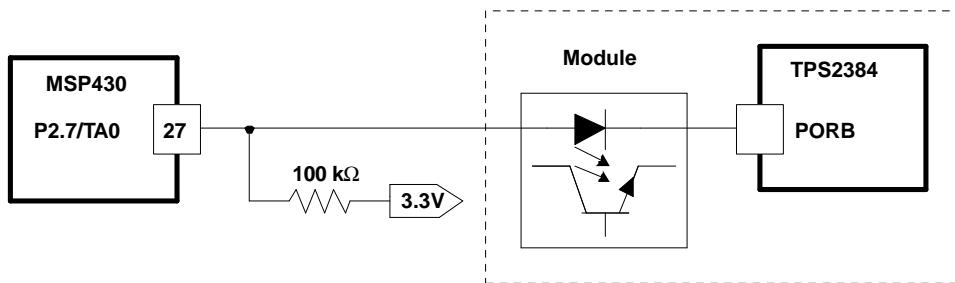
Figure 10. Power-On Reset Circuit Interface
