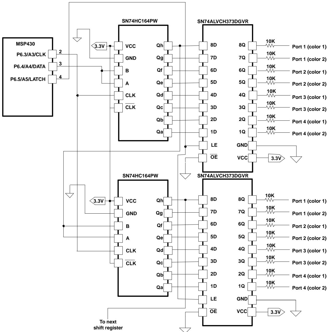
Figure 6. LED Interface Schematic
