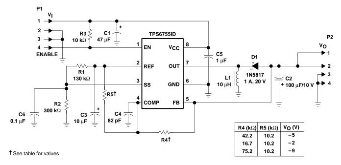
Figure 1. Application Circuit
