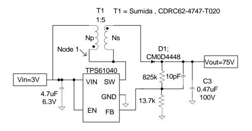
Figure 1. Application Circuit Using the TPS61040
