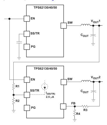
Figure 6. Ratiometric and Simultaneous Start Up Sequence
