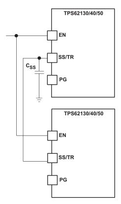
Figure 4. Ratiometric Start Up Using the SS/TR Pins
