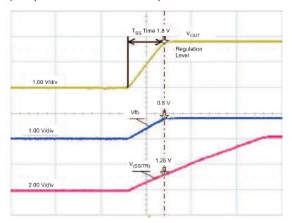
Figure 1. Soft Start Ramp Up Time
