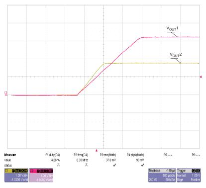
Figure 8. Ratiometric Start Up with  $V_{\text{out}}2$  Leading  $V_{\text{out}}1$
