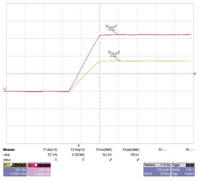
Figure 7. Ratiometric Start Up with V<sub>out</sub>1 Leading V<sub>out</sub>2
