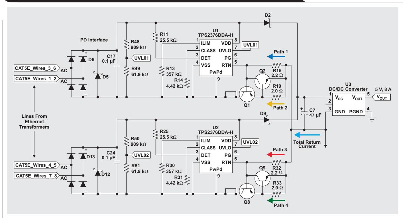
topology to provide an isolated 5 V at 8 A to the load.
