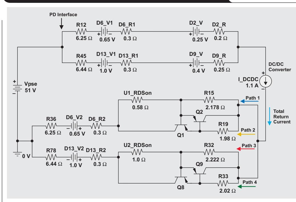
The values were adjusted so that all impedance mismatches were in one current loop, allowing for the largest imbalance. The four-pair architecture simulation previously discussed was run a second time to determine the extent of current imbalance in each current pair.
