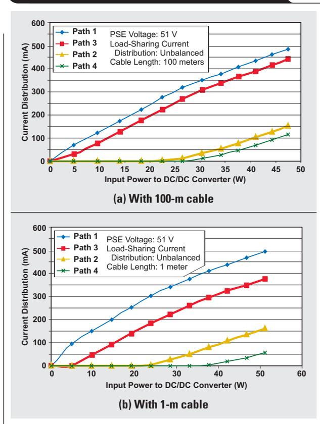
**Figure 8. Board-level test results of balanced current sharing**
