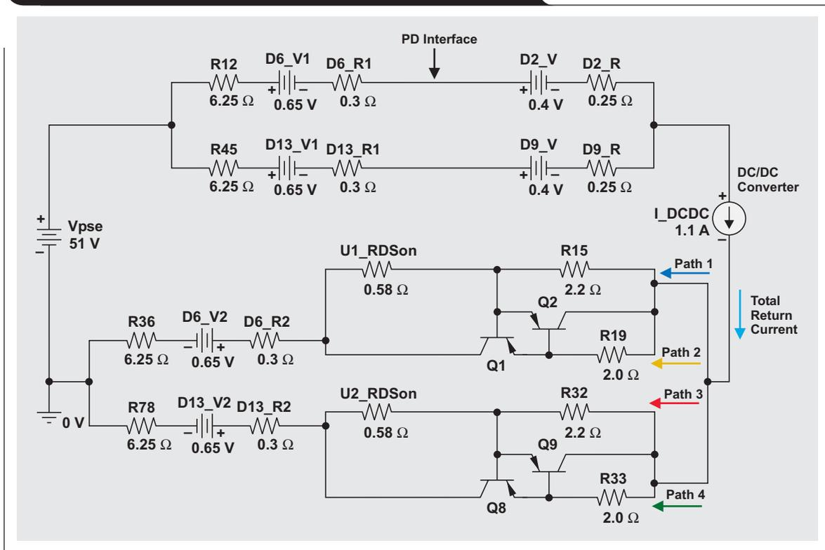
maximum of 100 m of Ethernet cable between the PD and PSE.<sup>1</sup> Figure 5 shows the simulation results for the corner areas of 100 m and 1 m of cable length when the model cable resistances (R12, R45, R36, R78) are modified. All simulations are done at the minimum PSE voltage of 51 V because input current is highest at this condition.
