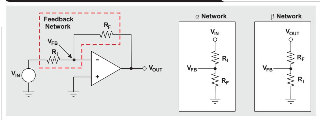
**Figure 6. Control-loop model of inverting op amp circuit**
