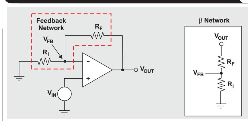
Figure 3 shows the control-loop model of the circuit in Figure 2. The parameter  $A_{OL}$  is the open-loop gain of the op amp and is always specified in any op amp data sheet. The control-loop model from Figure 3 can be used to express the closed-loop gain as
