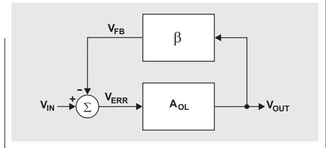
$A_{CL}(j\omega)$  is a complex function of the angular frequency,  $\omega$ . Also recall that to calculate the magnitude, both real and imaginary portions of the function need to be used in the same way that Equation 6 was obtained:
