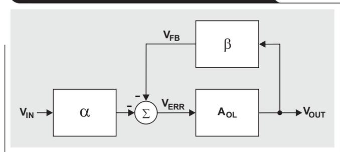
Assuming that there is a first-order response from the op amp, the complete closed-loop equations for the noninverting and inverting gain amplifiers are respectively represented by Equation 13 and Equation 18.
