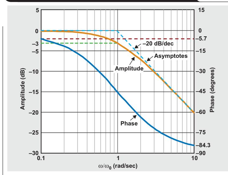
$\omega = \omega_0$ , the magnitude drops to  $1/\sqrt{2} = 0.707$ , or roughly  $-3$  dB. Above this frequency, the magnitude rolls off at a rate of  $-20$  dB/decade.
