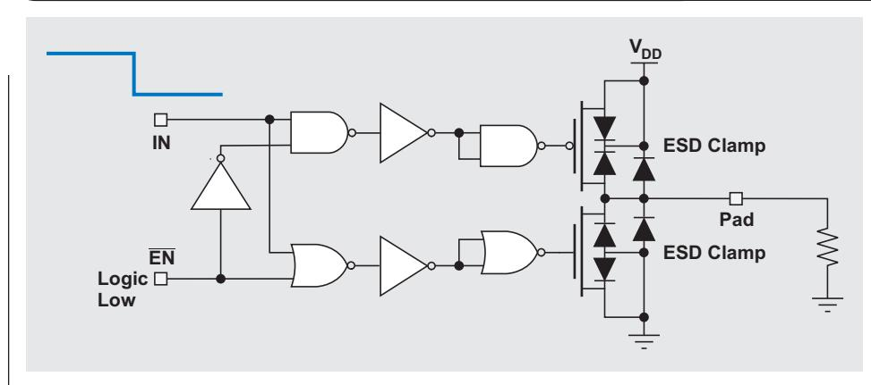
Figure 3 shows the proper test-circuit configuration for the transient falling edge of an output buffer. The resistor following the pad is usually  $50\ \Omega$ ; however, it can be a different value depending on the IC's requirements as stated in the product data sheet.
