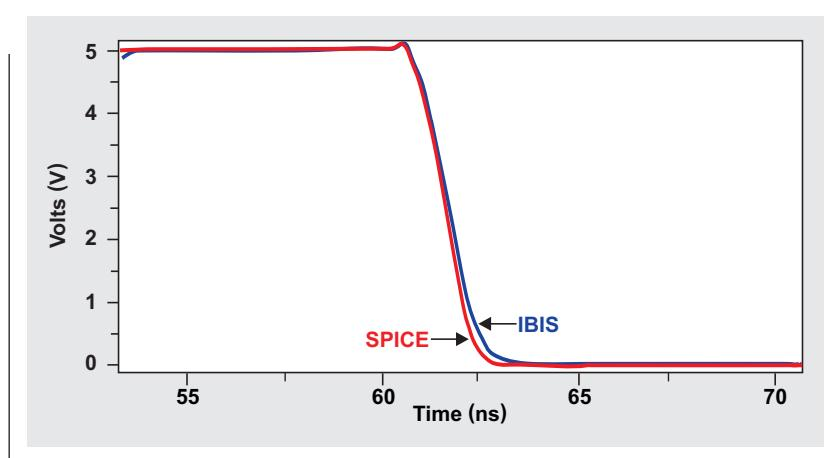
Figure 8 shows a similar fall-time comparison between the SPICE and IBIS models, also based on the ADS8319. Simulated model conditions were based on a 5-V power supply, a junction temperature of 25°C, and a typical process corner.
