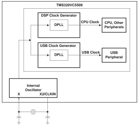
Figure 2. TMS320VC5509 USB Clock Generator
