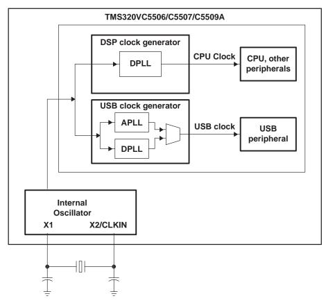
Figure 3. TMS320VC5506/C5507/C5509A USB Clock Generator
