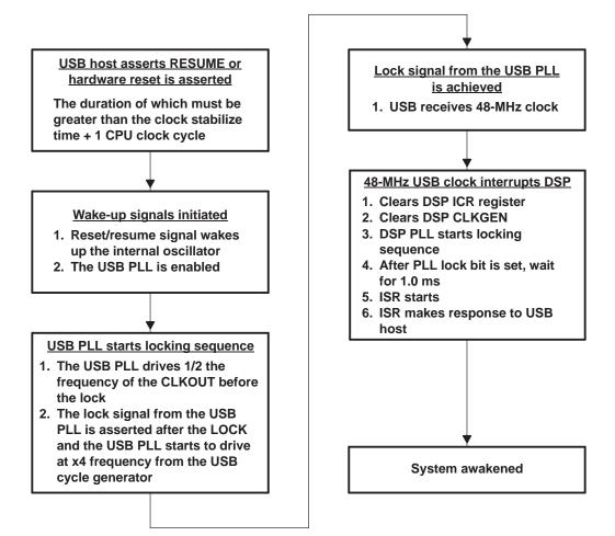
Figure 6. Waking Up the Internal Oscillator With a Hardware or USB Reset/Resume for the TMS320VC5509
