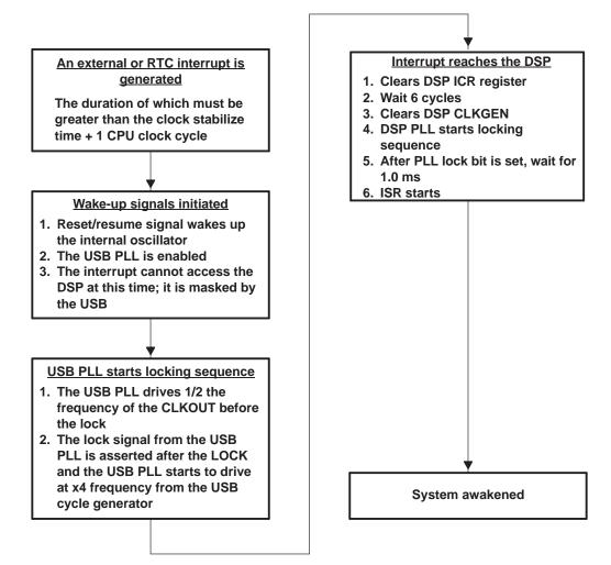
Figure 7. Waking Up the Internal Oscillator With an RTC or External Interrupt for the TMS320VC5506/C5507/C5509
