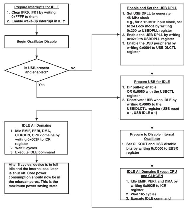
Figure 4. Disabling the Internal Oscillator on the TMS320VC5509
