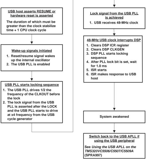
Figure 8. Waking Up the Internal Oscillator With a Hardware or USB Reset/Resume for the TMS320VC5506/C5507/C5509/C5509A
