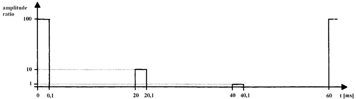
There are three clicks in the sequence each with different amplitudes. The amplitude ratio of the clicks is 100:10:1. Every click has a length of 100  $\mu$ s. The clicks will be emitted every 20 ms. Between two clicks there is a time of silence with a length of 19,9 ms (=20 ms-100  $\mu$ s). During this time the response signal of the click, i.e. the otoacoustic emissions, can be recorded.
