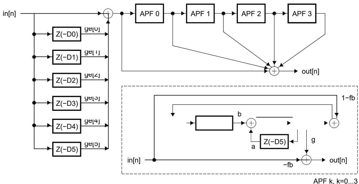
**Figure 12. Reverb Effect Block Diagram**
