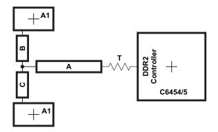
Figure 6. CK and ADDR\_CTRL Routing and Topology
