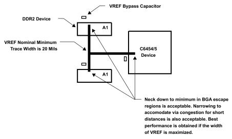
Figure 5. VREF Routing and Topology
