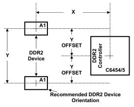
Figure 3. C6454/5 and DDR2 Device Placement
