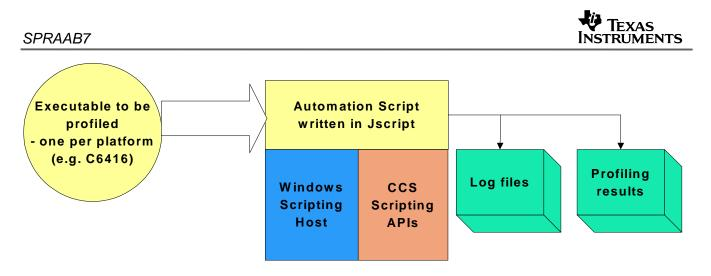
Figure 2. Flowchart of RF3 Profiling Test Bench
