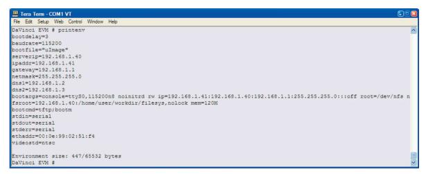
Figure 2. u-boot Environment for Booting Linux Kernel via Host TFTP
