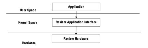
Figure 4.1. OMAP35x Resizer Interface Block-Diagram
