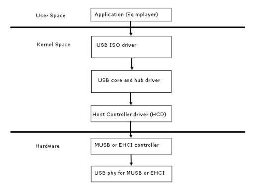
Figure 10.5. USB Driver: Illustration of ISO device Driver
