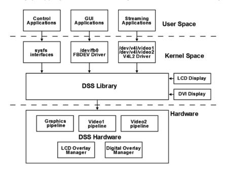
Figure 2.1. OMAP35x Display Subsystem Architecture
