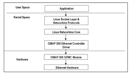
Figure 7.1. Linux Kernel Ethernet Driver
