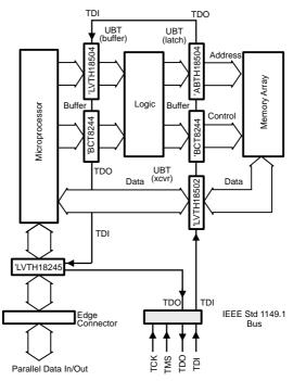
Figure 2-1. Boundary-Scan Testing Using the IEEE Std 1149.1 Bus
