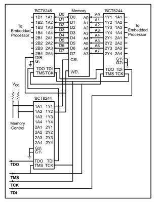
Figure 7-10. Block Diagram of Simplified Boundary-Scannable RAM Interface
