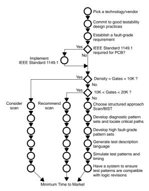
Figure 4-7. Testability Development Flow
