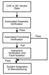
Figure 7-16. General Boundary-Scan Test
