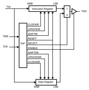
Figure 3-4. TAP Control Output Interconnect Diagram
