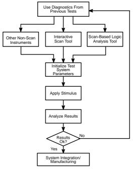
Figure 7-19. Interactive Verification and Fault Isolation
