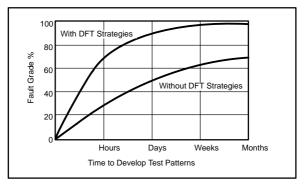
Figure 4-1. Fault Grade Versus Development Time
