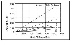
Figure 4-5. ASIC ppm Versus PCB ppm Rate
