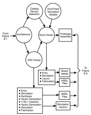
Figure 6-2. Designing Testability for ASICs and Boards
