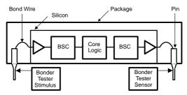
Figure 7-5. Bond-Wire Testing
