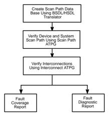
Figure 7-17. Assembly Verification Flow
