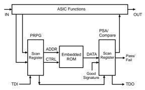
Figure 7-12. Testing Embedded ROM
