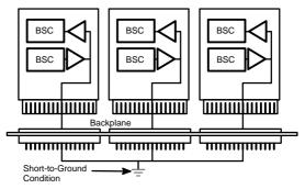
Figure 7-9. Backplane Short-to-Ground Fault
