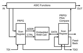
Figure 7-11. Testing Embedded RAM
