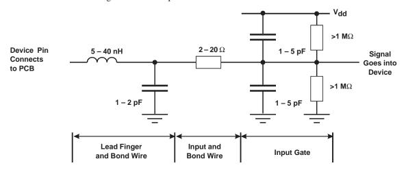
Figure 11. MOS Buffer Simplified Schematic
