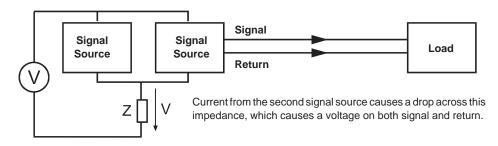
Common-mode noise is the noise voltage that travels down both the signal and return caused by a voltage drop across a shared impedance. Ground bounce on outputs is an example of common-mode noise.
