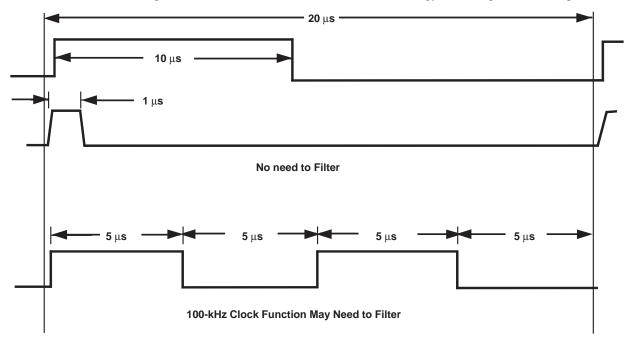
Figure 1. Signals Below 50 kHz Are Not EMI Concerns
