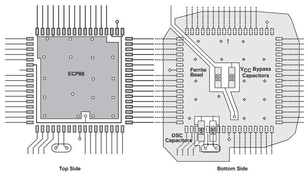
Figure 4. Microcomputer Ground
