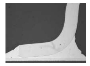
Figure 16. Sn/Ag/Cu Solder (235°C Peak), 1000 Temperature Cycles
