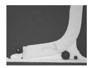
Figure 21. Sn/Zn Solder, 1000 Temperature Cycles
