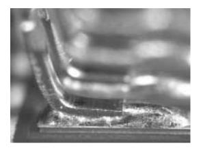
Figure 9. Sn/Bi Paste, SSOP Package
