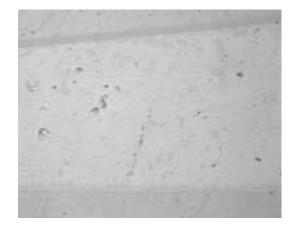
Figure 31. Sn/Ag/Cu/Sb Solder, 1000 Temperature Cycles
