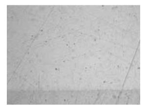
Figure 30. Sn/Ag/Cu/Sb Solder, 0 Temperature Cycles
