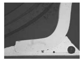
Figure 20. Sn/Zn/Bi Solder, 1000 Temperature Cycles
