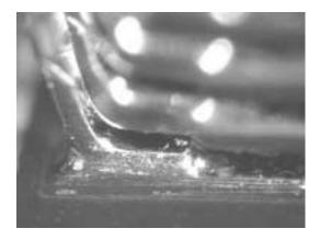
Figure 6. Sn/Pb/Ag Control Paste, SSOP Package
