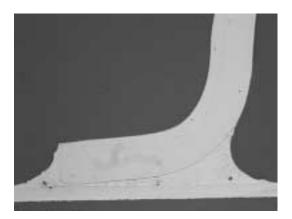
Figure 15. Sn/Pb/Ag Solder, 1000 Temperature Cycles
