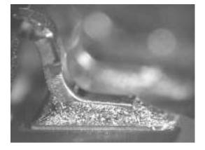
Figure 11. Sn/Zn/Bi Paste, SOIC Package
