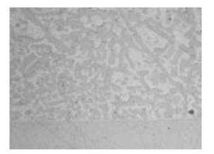
Figure 28. Sn/Bi Solder, 0 Temperature Cycles
