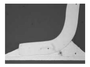
Figure 18. Sn/Bi Solder, 1000 Temperature Cycles
