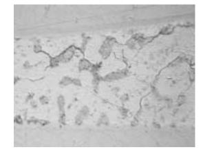
Figure 23. Sn/Pb/Ag Solder, 1000 Temperature Cycles
