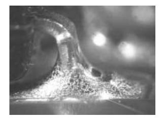
Figure 36. Sn/Ag/Cu Alloy Paste (235°C Peak), Figure 37. Sn/Ag/Cu Alloy Paste (260°C Peak), Ni/Pd/Au-Finished SOIC Package Ni/Pd/Au-Finished SOIC Package
