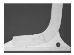
Figure 19. Sn/Ag/Cu/Sb Solder, 1000 Temperature Cycles
