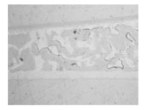
Figure 29. Sn/Bi Solder, 1000 Temperature Cycles
