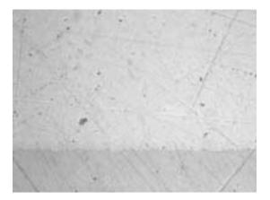
Figure 24. Sn/Ag/Cu Solder (235°C Peak), 0 Temperature Cycles
