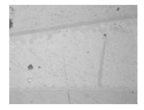
Figure 27. Sn/Ag/Cu Solder (260°C Peak), 1000 Temperature Cycles
