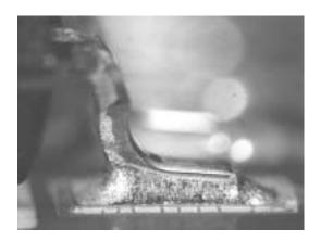
Figure 8. Sn/Ag/Cu Paste (260°C Peak), SOIC Package
