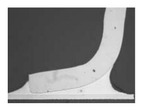
Figure 17. Sn/Ag/Cu Solder (260°C Peak), 1000 Temperature Cycles
