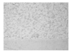
Figure 22. Sn/Pb/Ag Solder, 0 Temperature Cycles
