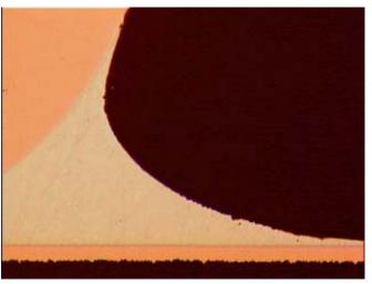
Figure 29. Group 3B, NiPd Finish, Stored in Tubes, 96-h Exposure
