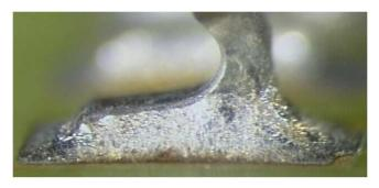
Figure 12. Group 1A, NiPdAu Finish, Stored Loose, 96-h Exposure
