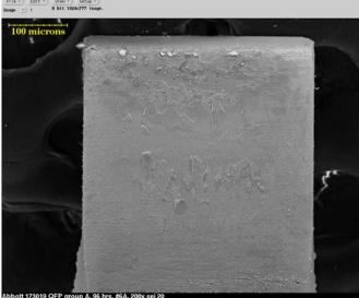
Figure 8. Group 6A NiPdAu 0.02- $\mu$ m (0.8- $\mu$ ") Pd, Loose, 96 h, 25×
