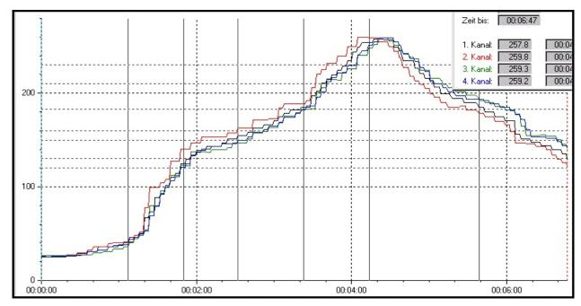
Figure 10. Reflow Profile Used for 20-Pin SOIC Units
