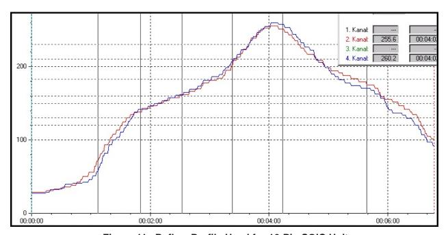
Figure 11. Reflow Profile Used for 16-Pin SOIC Units
