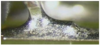
Figure 19. Group 4B, Sn Finish, Stored in Tubes, 96-h Exposure
