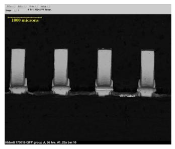
Figure 2. Group 1A NiPdAu 0.01-μm (0.4-μ") Pd, Loose, 96 h, 25×, Bottom Lead View
