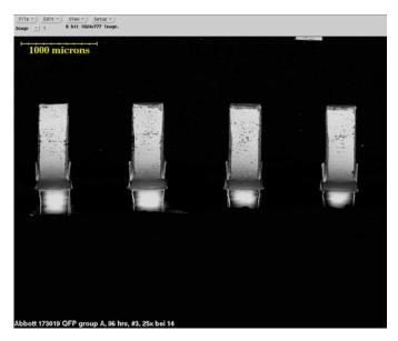
Figure 6. Group 3A NiPdAu 0.02- $\mu$ m (0.8- $\mu$ ") Pd, Loose, 96 h, 25×
