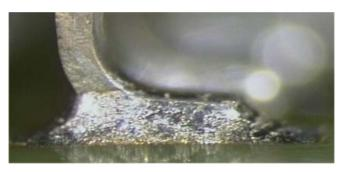
Figure 14. Group 2A, NiPdAu Finish, Stored Loose, 96-h Exposure
