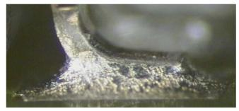
Figure 13. Group 1B, NiPdAu Finish, Stored in Tubes, 96-h Exposure
