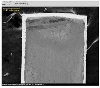
Figure 3. Group 1A NiPdAu 0.01- $\mu$ m (0.4- $\mu$ ") Pd, Loose, 96 h, 200×
