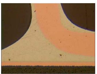
Figure 30. Group 4A, Sn Finish, Stored Loose, 96-h Exposure
