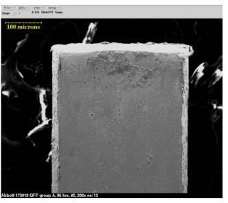
Figure 5. Group 2A NiPdAu 0.02- $\mu$ m (0.8- $\mu$ ") Pd, Loose, 96 h, 200×
