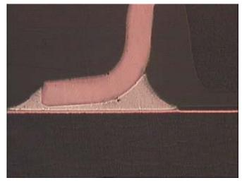
Figure 24. Group 1A, NiPdAu Finish, Stored Loose, 96-h Exposure
