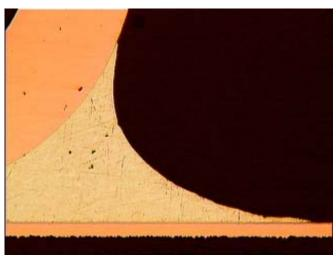
Figure 25. Group 1B, NiPdAu Finish, Stored in Tubes, 96-h Exposure
