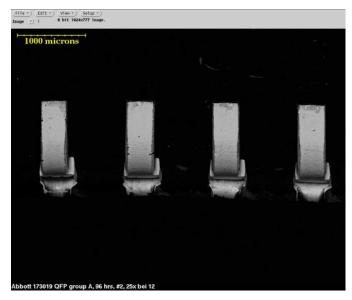
Figure 4. Group 2A NiPdAu 0.02-μm (0.8-μ") Pd, Loose, 96 h, 25×
