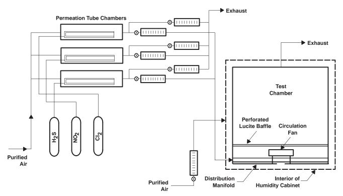
Figure 1. Schematic of MFG Chamber
