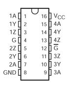
Figure 4-1. N Package (Top View)
