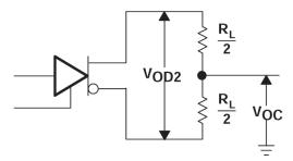
Figure 6-1. Differential and Common-Mode Output Voltages
