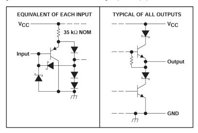
Figure 7-1. Schematics of Inputs and Outputs
