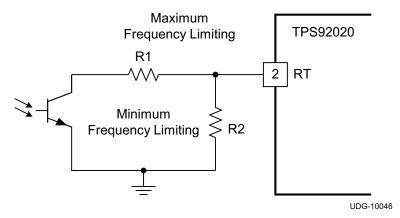
Figure 18. Maximum and Minimum Frequency Setting for TPS92020
