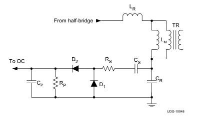
Figure 20. Current Sensing for LLC Resonant Converter
