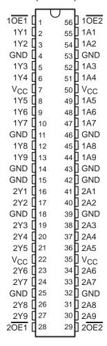
The 74ACT16825 is packaged in TI's shrink small-outline package, which provides twice the I/O pin count and functionality of standard small-outline packages in the same printed-circuit-board area.
