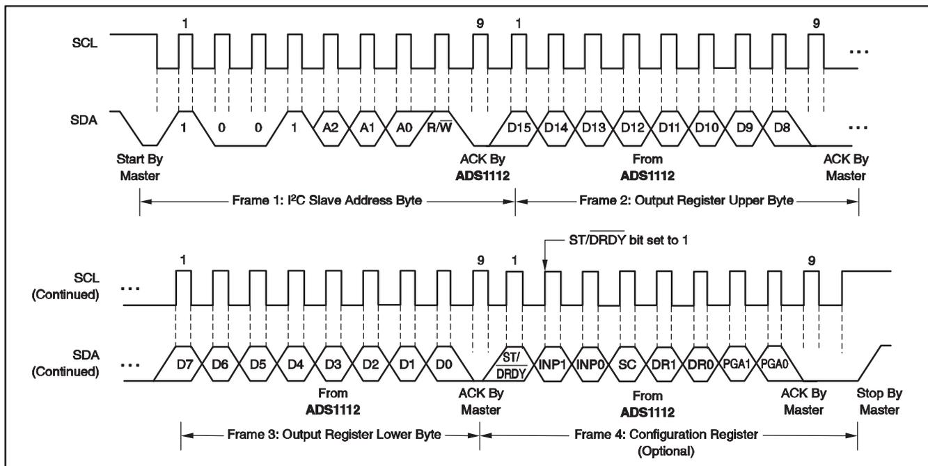
Figure 2. Timing Diagram for Reading From the ADS1112
