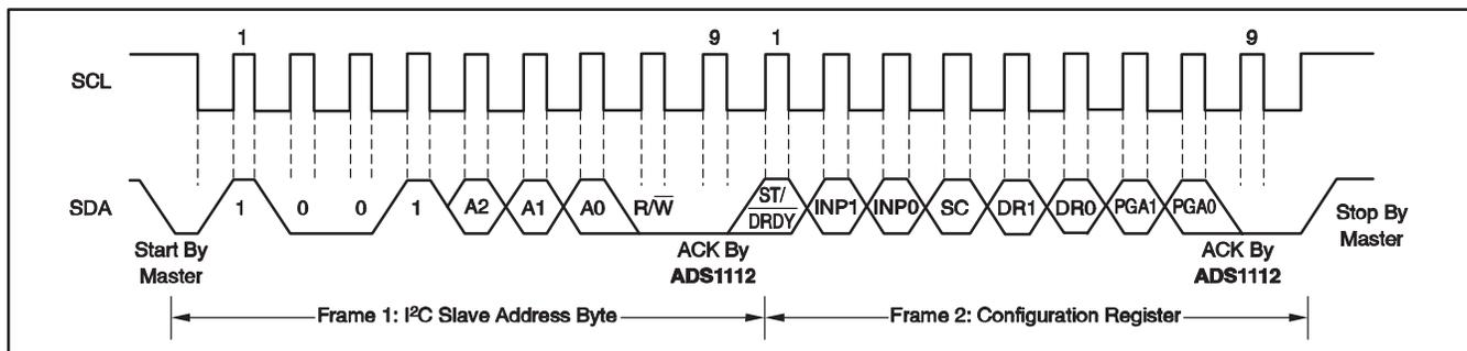
Figure 3. Timing Diagram for Writing To the ADS1112
