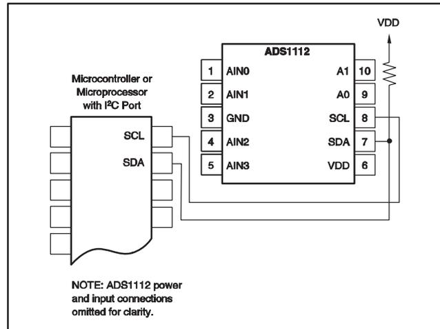
Figure 7. Using GPIO with a Single ADS1112
