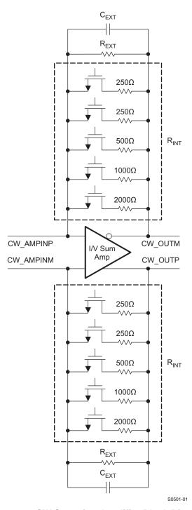
Figure 86. CW Summing Amplifier Block Diagram
