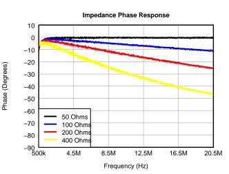
Figure 11. Input Impedance With Active Termination (Phase)
