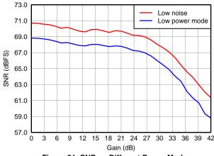
Figure 30. SNR, LNA = 18 dB and Low Power Mode
