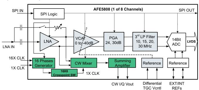
Figure 63. Functional Block Diagram
