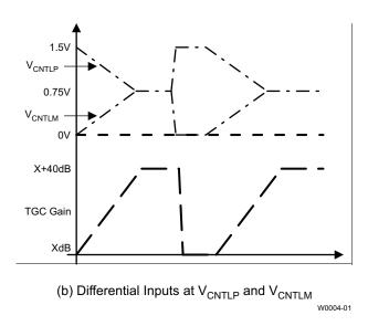
Figure 85. V<sub>CNTLP</sub> and V<sub>CNTLM</sub> Configurations
