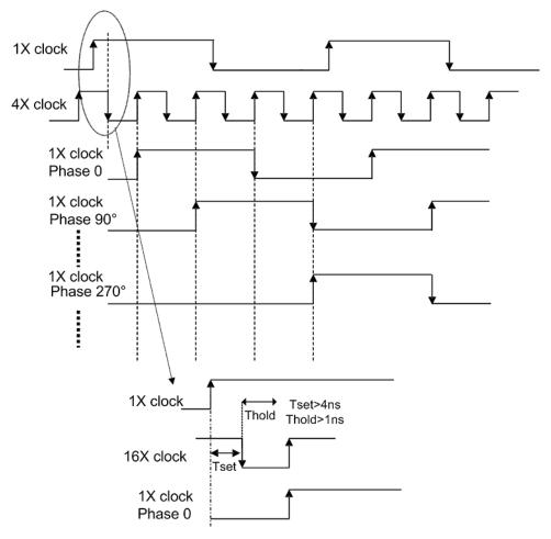
Figure 74. 8 x  $f_{cw}$  and 4 x  $f_{cw}$  Timing Diagram
