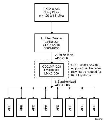
Figure 90. ADC Clock Distribution Network
