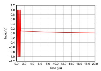
Figure 53. Pulse Inversion Asymmetrical Positive Input
