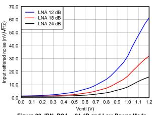
Figure 22. IRN, PGA = 24 dB and Low Power Mode
