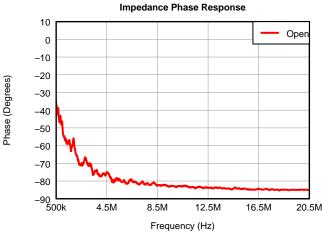
Figure 9. Input Impedance Without Active Termination (Phase)
