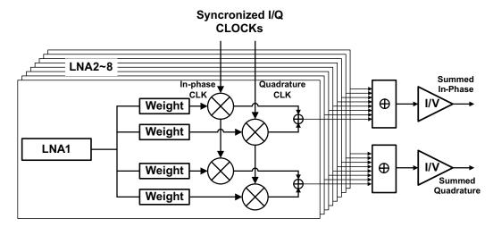
Figure 75. Block Diagram of 1 x  $f_{cw}$  mode
