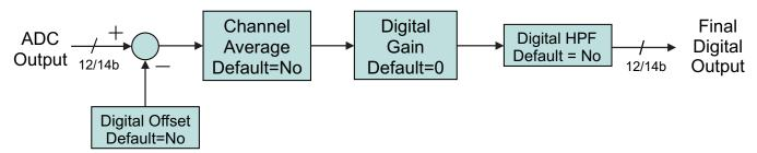
Figure 62. ADC Digital Block Diagram
