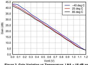
Figure 3. Gain Variation vs Temperature, LNA = 18 dB and PGA = 24 dB
