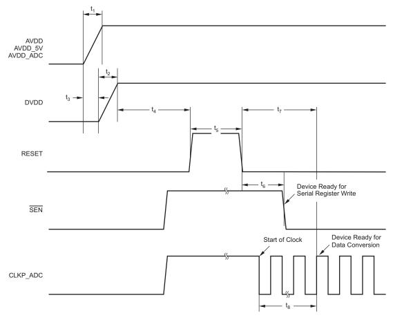
10  $\mu$ s <  $t_1$  < 50 ms, 10  $\mu$ s <  $t_2$  < 50 ms, -10 ms <  $t_3$  < 10 ms,  $t_4$  > 10 ms,  $t_5$  > 100 ns,  $t_6$  > 100 ns,  $t_7$  > 10 ms, and  $t_8$  > 100  $\mu$ s.
