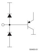
Figure 77. Equivalent Circuits of V<sub>CNTLP/M</sub>
