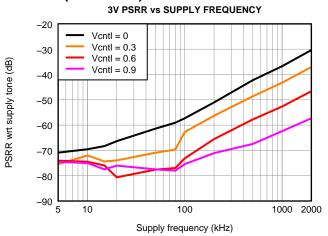
Figure 49. AVDD Power Supply Rejection Ratio, 100 mV<sub>PP</sub> Supply Noise With Different Frequencies
