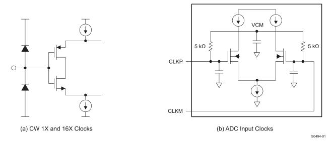
Figure 78. Equivalent Circuits of Clock Inputs
