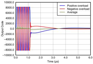
Figure 54. Pulse Inversion Asymmetrical Negative Input
