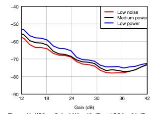
Figure 40. HD3 vs Gain, LNA = 12 dB and PGA = 24 dB and  $V_{OUT}$  = -1 dBFS
