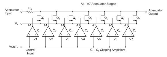
Figure 65. Simplified Voltage Controlled Attenuator (Analog Structure)
