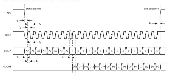
Figure 60. Serial Interface Register Read
