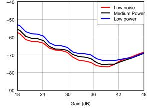
Figure 42. HD3 vs Gain, LNA = 18 dB and PGA = 24 dB and  $V_{OUT}$  = -1 dBFS
