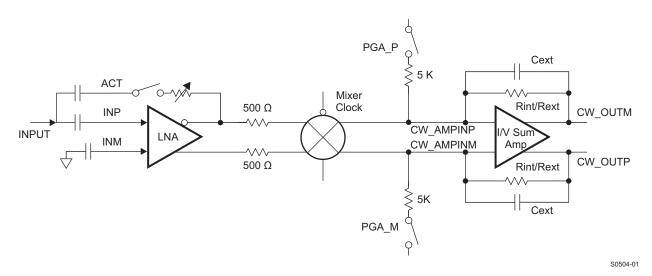
Figure 91. AFE5808 PGA Test Mode
