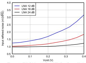
Figure 21. IRN, PGA = 24 dB and Medium Power Mode
