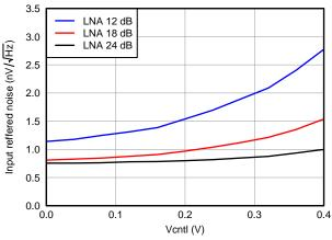
Figure 19. IRN, PGA = 24 dB and Low Noise Mode
