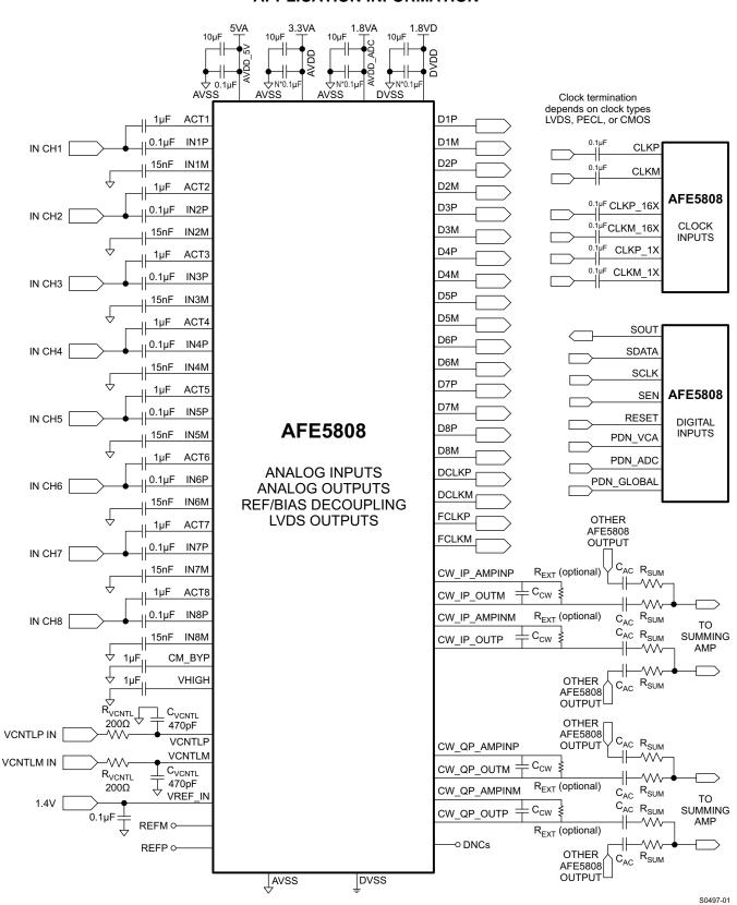
Figure 81. Application Circuit
