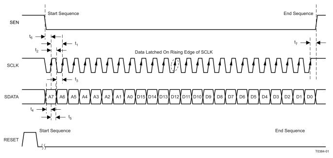
Figure 59. SPI Timing
