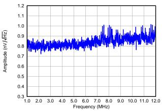
Figure 26. ORN, PGA = 24 dB and Low Power Mode
