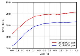
Figure 28. ORN, PGA = 24 dB and Low Noise Mode
