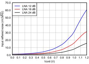
Figure 20. IRN, PGA = 24 dB and Medium Power Mode
