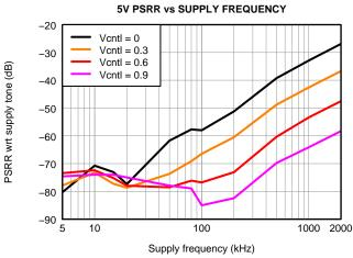
Figure 50. AVDD\_5V Power Supply Rejection Ratio, 100 mV<sub>PP</sub> Supply Noise With Different Frequencies
