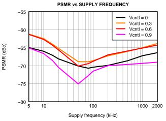
Figure 48. AVDD\_5V Power Supply Modulation Ratio, 100 mV<sub>PP</sub> Supply Noise With Different Frequencies
