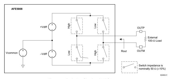
Figure 80. Equivalent Circuits of LVDS Outputs
