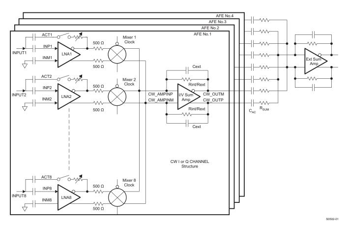
Figure 87. CW circuit with Multiple AFE5808s
