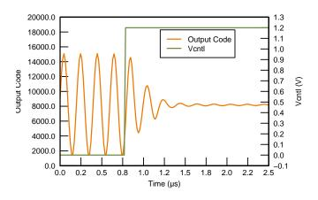
Figure 52. V<sub>CNTL</sub> Response Time, LNA = 18 dB and PGA = 24 dB
