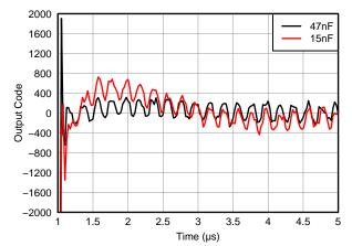
Figure 57. Overload Recovery Response vs INM capacitor(Zoomed), V $_{\rm IN}$  = 50 mVpp/100  $\mu$ V $_{\rm PP}$ , Max Gain
