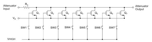
Figure 66. Simplified Voltage Controlled Attenuator (Digital Structure)
