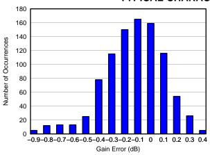
Figure 6. Gain Matching Histogram, VCNTL = 0.9 V (936 channels)
