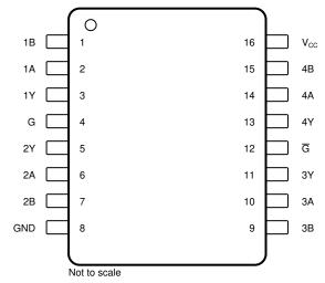
Figure 5-1. D, J, N, NS, and PW Package 16-Pin SOIC, CDIP, PDIP, SO, and TSSOP (Top View)
