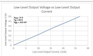
Figure 6-2. Low-Level Output Voltage vs Low-Level
