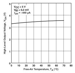
Figure 9-2. High-Level Output Voltage vs Free-Air Temperature
