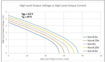
Figure 6-1. High-Level Output Voltage vs High-Level Output Current
