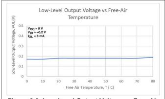
Figure 6-3. Low-Level Output Voltage vs Free-Air Temperature
