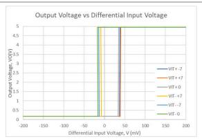
Figure 6-8. AM26LS32A Output Voltage vs Differential Input Voltage
