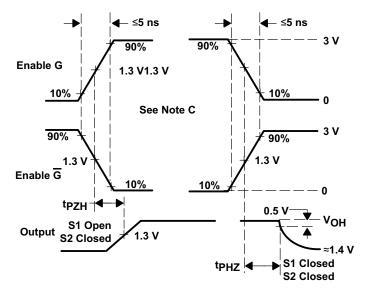
Figure 7-3. Voltage Waveforms For t<sub>PHZ</sub>, t<sub>PZH</sub>
