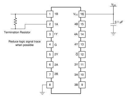
Figure 9-3. Layout with PCB Recommendations
