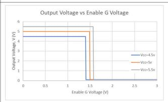
Figure 6-6. Output Voltage vs Enable G Voltage
