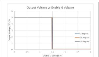
Figure 6-7. Output Voltage vs Enable G Voltage
