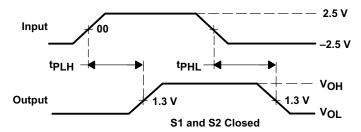
Figure 7-2. Voltage Waveforms For t<sub>PLH</sub>, t<sub>PHL</sub>
