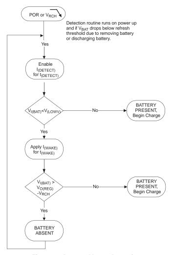
Figure 7. Battery Absent Detection
