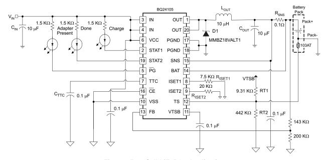
Figure 15. 1-Cell LiFePO4 Application
