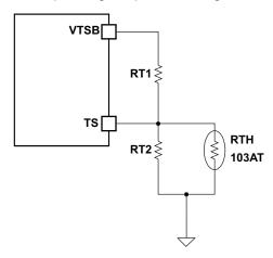
Figure 13. TS Resistor Network
