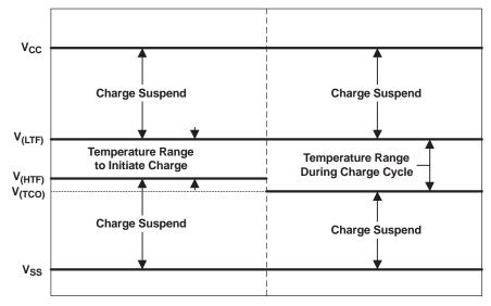
Figure 6. TS Pin Thresholds
