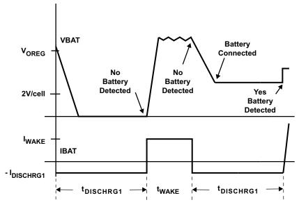
Figure 8. Battery Detect Timing Diagram
