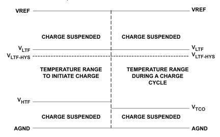
Figure 32. TS, Thermistor Sense Thresholds
