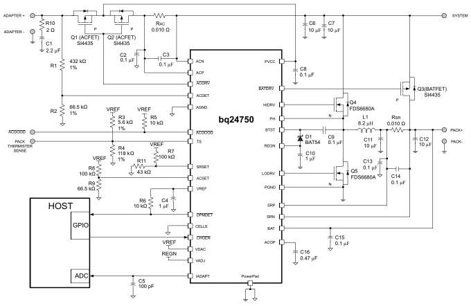
A. V<sub>IN</sub>= 20 V, V<sub>BAT</sub> = 3-cell Li-Ion, I<sub>CHARGE</sub> = 3 A, I<sub>ADAPTER\_LIMIT</sub> = 4 A, T<sub>BAT</sub> = 0-45°C
