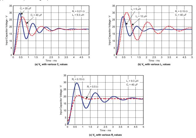
Figure 38. Parametric Study Of The Input Voltage
