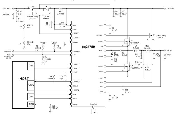
A.  $V_{IN}$ = 20 V,  $V_{BAT}$  = 3-cell Li-lon,  $I_{CHARGE}$  = 3 A,  $I_{ADAPTER\_LIMIT}$  = 4 A,  $T_{BAT}$  = 0-45°C
