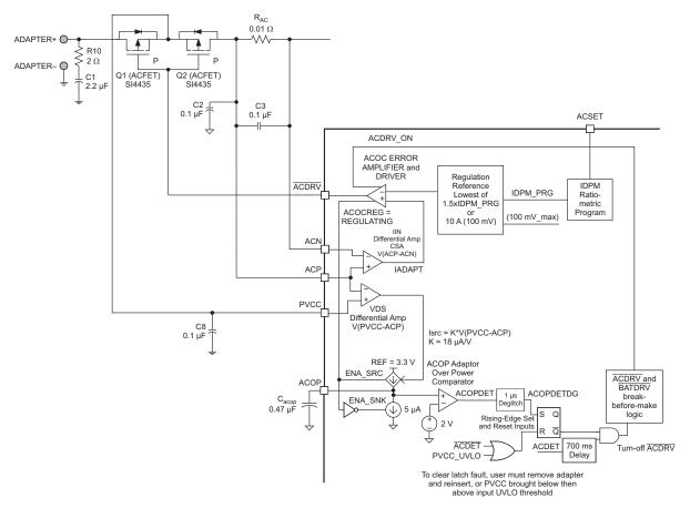
Figure 36. ACOC / ACOP Circuit Functional Block Diagram
