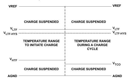
Figure 32. TS, Thermistor Sense Thresholds
