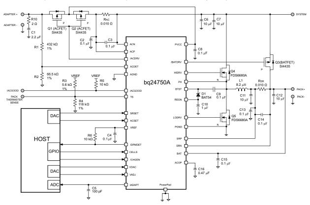
A.  $V_{IN}$ =20 V,  $V_{BAT}$  = 3-cell Li-Ion,  $I_{CHARGE}$  = 3 A,  $I_{ADAPTER\_LIMIT}$  = 4 A,  $T_{BAT}$  = 0-45°C
