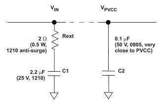
Figure 39. Recommended Input Filter Design
