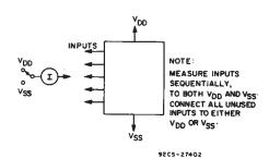
Fig. 14-Input current test circuit.
