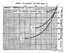
Fig. 6—Typical p-channel output high (source) current characteristics.
