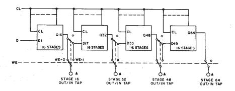
Fig. 1—CD4517B functional block diagram (one half).
