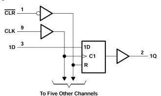
Figure 7-1. Logic Diagram (Positive Logic)
