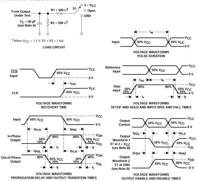
Figure 6-1. Load Circuit and Voltage Waveforms
