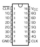
Figure 4-1. D or N Package (Top View)
